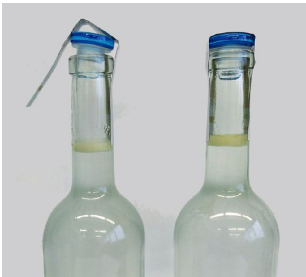
Example of overpressure test results
